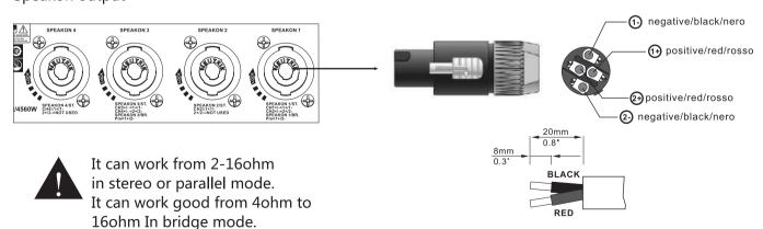
We don't suggest you use the amplifier under 40hm bridge mode, it will short its normally use life or have some Unnecessary failure.
